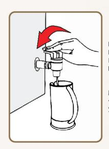
Push to lock for continuous flow. Return the lever to stop. If lever does not lock, rotate it 180° before dispensing.
